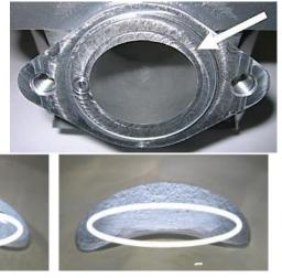
The exhaust port may show partial manual grinding done by the manufacturer to eliminate minor casting defects and/or to eliminate the NIKASIL burr at the end of the NIKASIL plating (see above right picture).
