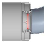
A steel ball with 28.0mm diameter **must not** pass through Section "A" and
