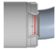
A steel ball with a 28.0mm diameter **must not** pass through Section "A" and
