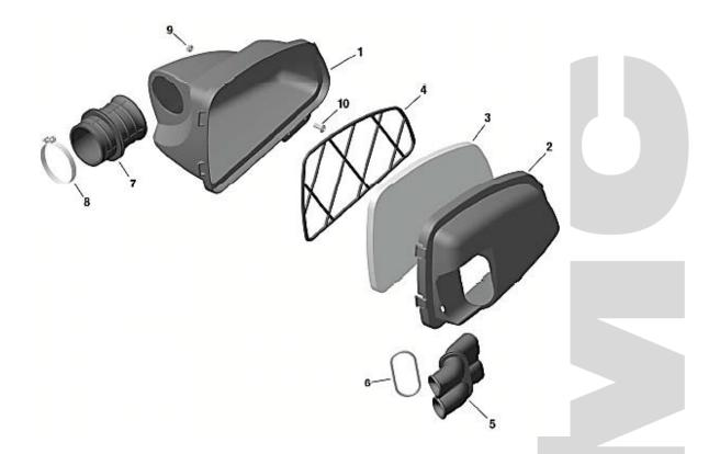
At intake silencer cover (Pos 2, Rotax 225022), it is mandatory to fit the O-ring (Pos 6) on the intake silencer tube (Pos 5). Intake silencer tube (Pos 5) and carburettor socket (Pos 7) are marked with the wording "ROTAX".
