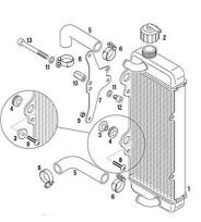
The support plate (Pos 7) enables two different mounting Positions (height) of the radiator. Both mounting Positions are legal to be used.
