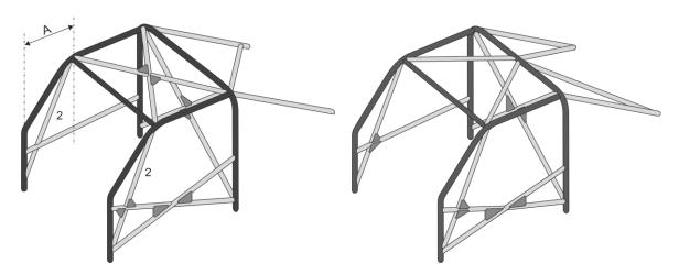
17.3. Places (marked red in picture), where the driver's helmet can come into contact with the safety cage during an accident, must be covered with a padding in accordance with FIA 8857-2001 standard. Padding must be fixed tightly to the safety cage bar, with no possibility to move it or to turn it on the radius of the bar.
