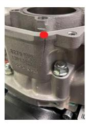
Example 2, Exhaust valve flange area repair.
